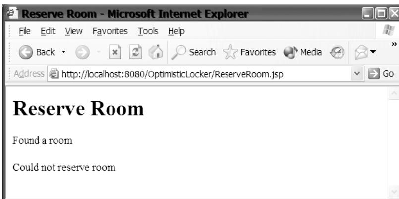
Figure 8-13. The second thread is unable to reserve the room, even though it found the available room.
